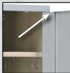
STANDARD Marquis Student Lockers include a 3" wide 18 gauge full height door stiffener spot welded to the inner door face and MIG welded to the hinge side as well as to the top and bottom door flanges providing a rigid torque-free door. A 1-1/2" wide stiffener will be furnished for 9" wide Marquis doors.
