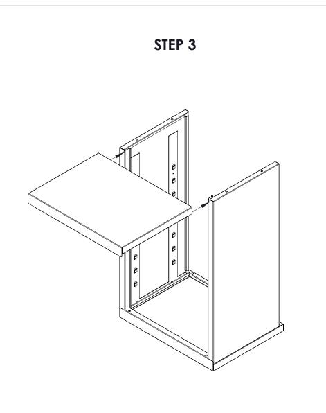
3. Insert top/bottom part sliding it into the side panels
