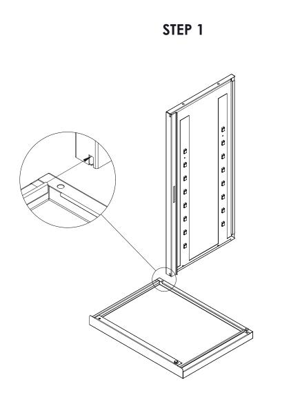
1. Insert side panel into the bottom/top hem and slide until it bumps with the front.
