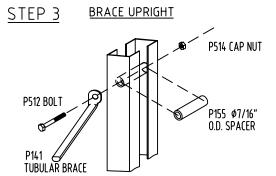
SET GATE ON FLOOR IN UPRIGHT POSITION AND EXTEND GATE TO ENABLE PLACEMENT OF \$\phi7/16\ O.D. SPACER BETWEEN PICKET CHANNELS. HOLDING THE SPACER IN PLACE, THREAD TUBULAR BRACE, PICKET CHANNELS, AND SPACER WITH \$\phi5/16 \times 1-3/4" HEX HEAD CAP BOLT AND SECURE WITH \$\phi5/16" CAP NUT.
